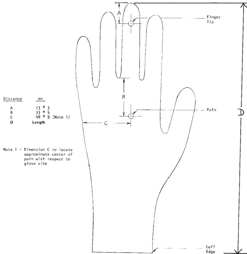
FIG. 1 Location of Thickness and Length Measurements
